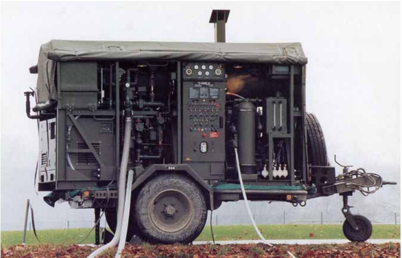
**Mobile steam desalination plant, mobile on a trailer towed by truck; supplied to the Italian Army for the foreign missions of the Armed Forces.**
