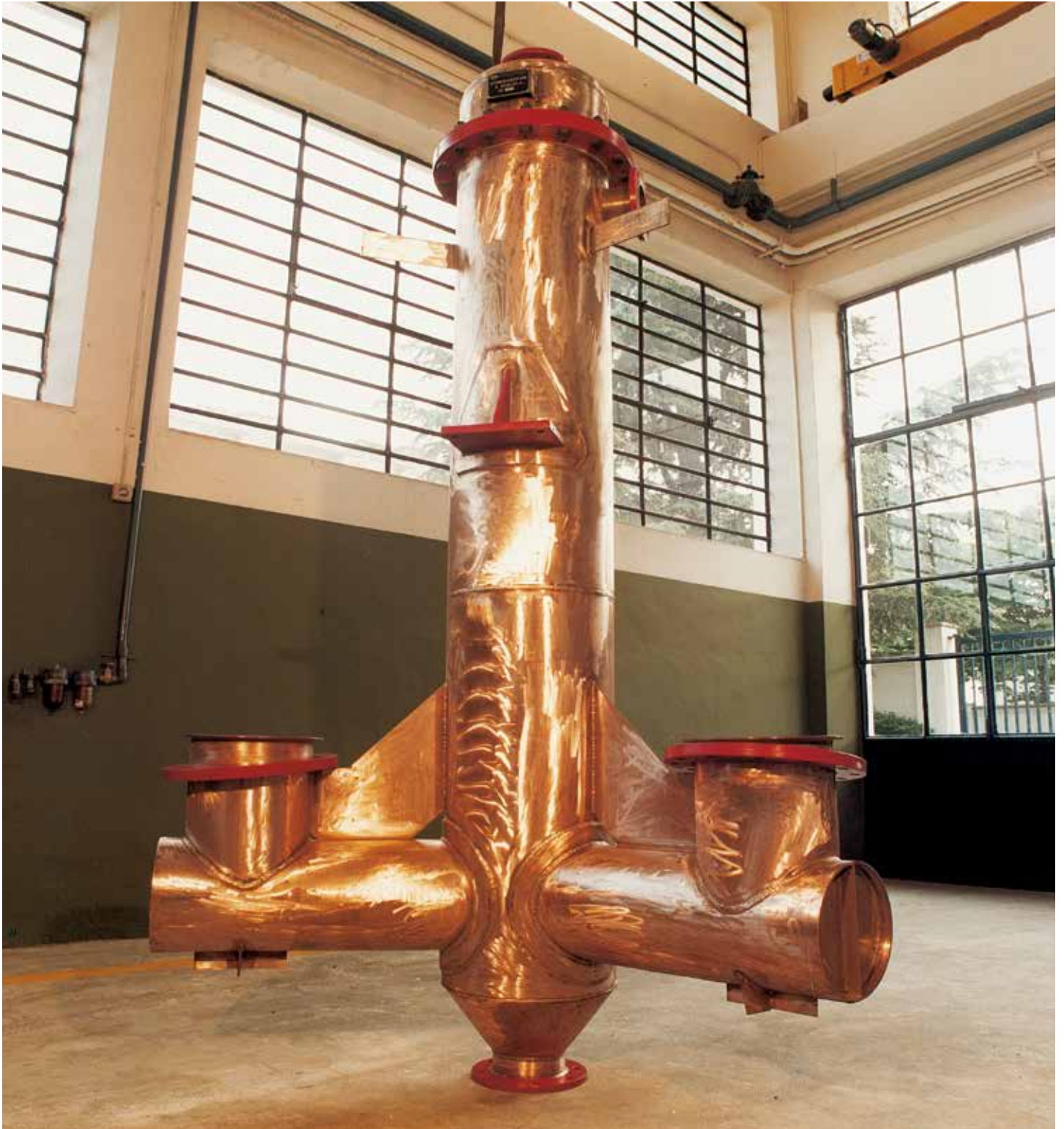
Direct contact condenser for vacuum unit
