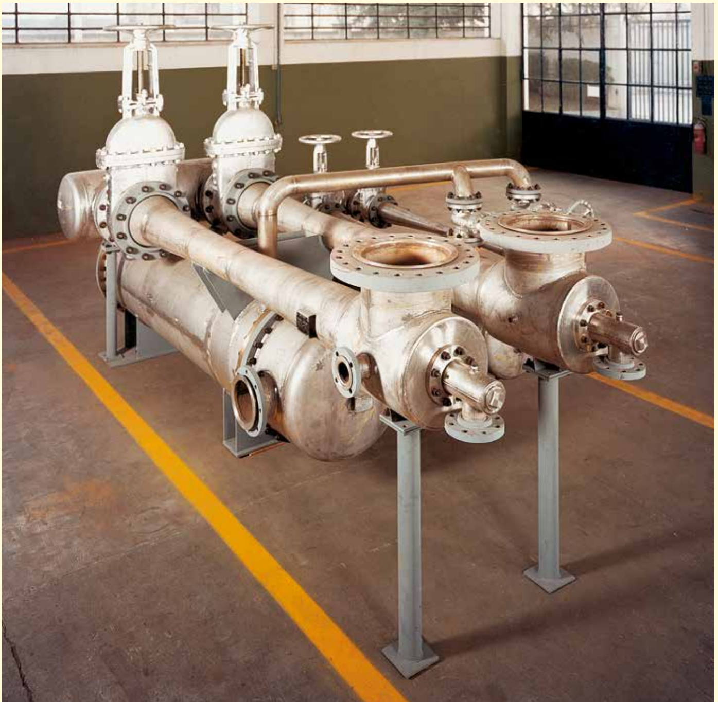
Two-stage twin element vacuum group with separate inter-after condenser
